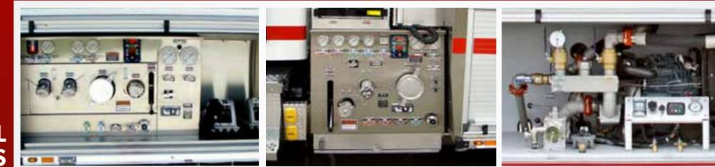
Choose the pump panel location that best fits your needs. Pump controls can be in the driver front compartment for PTO pumps, side or top mounted, or compartment mounted for portable pumps.
