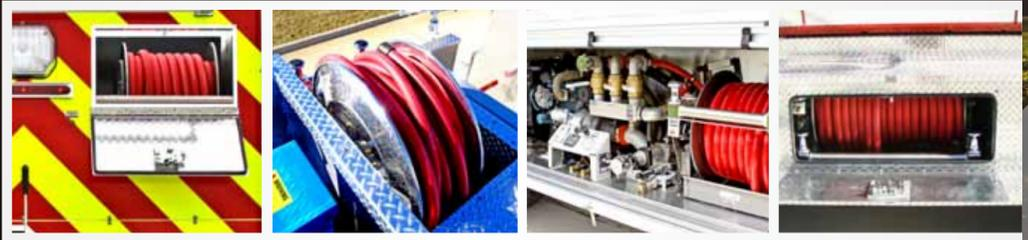
Booster reels can be notched in the upper rear corner of the tank with a hinge down door, above the pump in the dunnage area or in front of the hose bed, in any compartment specified by the department or under the cab depending on the chassis.
