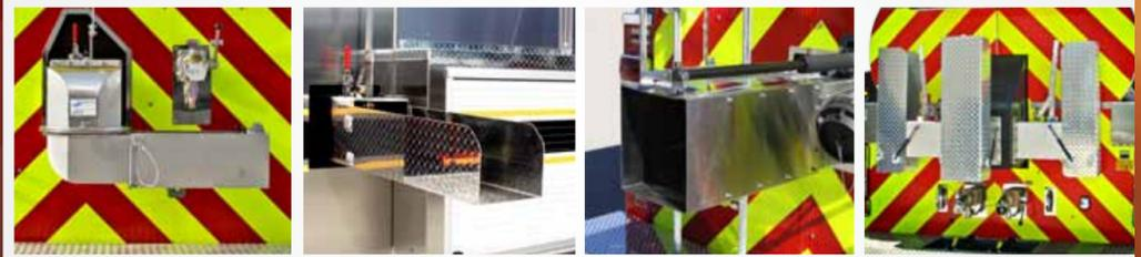
Engineered for the needs of your department, Toyne offers multiple dump chute options. Choose from stainless steel swivel dump, stainless steel dump valve with aluminum hinged chute, or stainless steel dump valve with electric chute and valve with option for in-cab controls. Toyne fire apparatus can also be outfitted with a three chute manifold system for the rear of the body.
