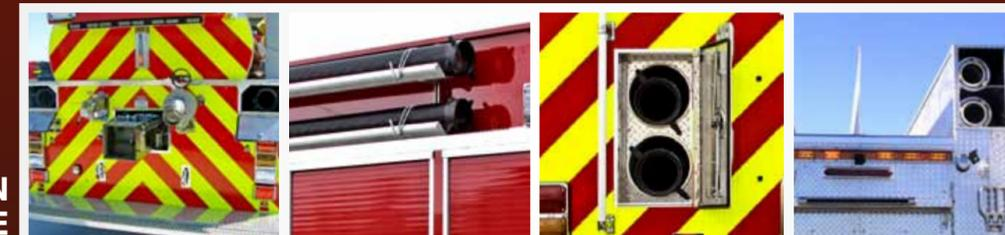
When drafting becomes necessary, it's critical for your hard suction hoses to be right at hand. Toyne offers hard suction storage options enclosed above the low side compartment, exterior mounted above each high side or low side compartment, slide-in from the rear or enclosed above the high side compartments.
