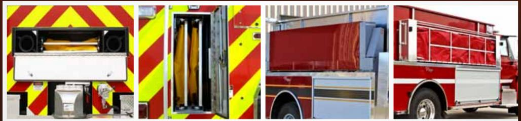
Toyne Tailored Apparatus are designed to hold 1000-3500 gallon portable tanks with steel or aluminum frames. Storage options include slide-in through tank, slide-in on edge, a Zico hydraulic rack with optional covering or manual portable tank racks.
